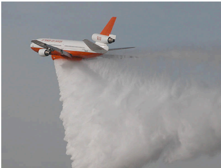
Figure 10.C13 Tanker 910 dropping water over the Victorville Airport during a demonstration for Los Angeles County Fire officials on 15 December 2006. Tanker 910 is a converted McDonnell Douglas DC-10 that can carry up to 12,000 gallons (45,000 l) of water or fire retardant and release it in 8 s. (source: Wikipedia)
