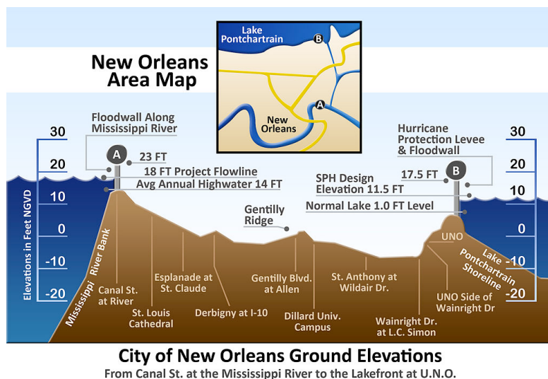
Figure 15.C2 Vertical cross-section of New Orleans, showing maximum levee height of 7 m (23 ft). Vertical scale exaggerated. New Orleans lies below sea level and has to be protected by levees and pumps against the ocean (right; Lake Pontchartrain) but also against the Mississippi River (left). (source: Wikipedia/NASA)
